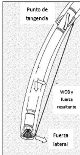
Figura 4.7.0.1: Montaje pendular [42]
