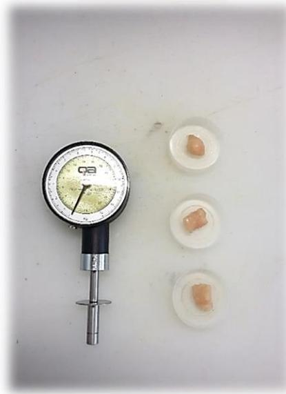
**Figura 31.** Penetrómetro, fruit pressure tester. Modelo FT327
