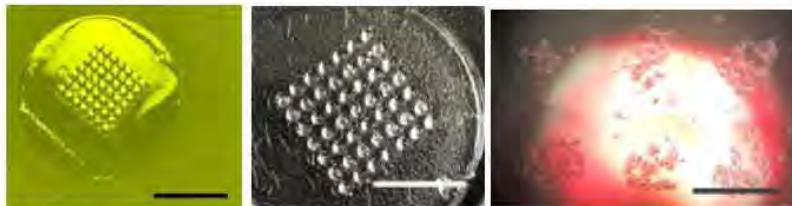
Figure 9. Polyacrylamide hydrogels with well structures a), vertical pillars b) and A549 cells seeded on 300 micron wide hydrogel pillars c). (scale bars are 1 cm for a and b; 300 µm for c).
