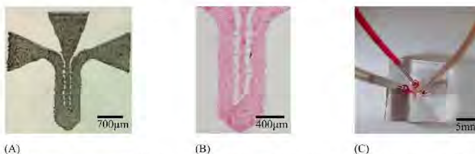
Figure 6. A) Laser micropatterned PMMA mold for 2-input 2-output microfluidic channel design. B) Example of colorant microfluidics inside PDMS microchannel for bonding validation. C) Microfluidic device.
