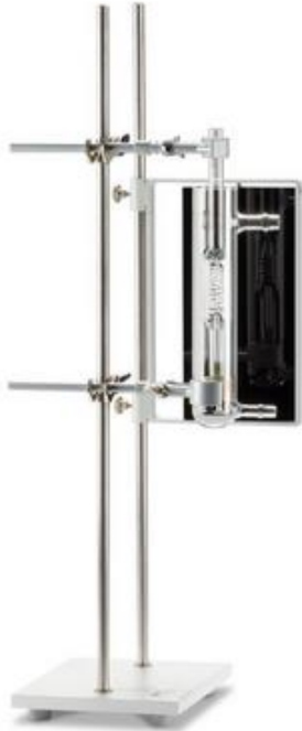
Figura 10 Suppository testing SSP (41)
