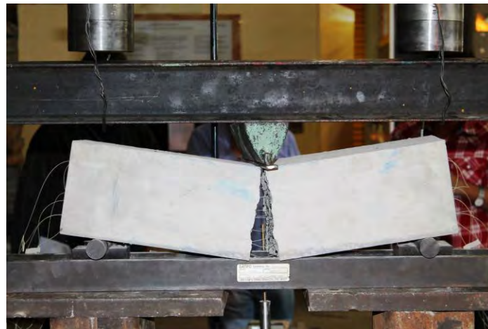
Figure 7. Flexural concrete beam with embedded thick optical fibers after failure.
