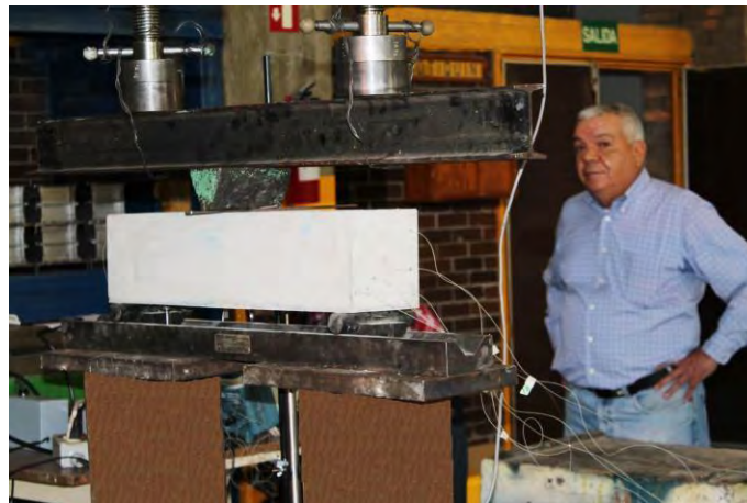
Figure 5. Reinforced concrete beam with the embedded optical fibers installed at the mechanical test facility.
