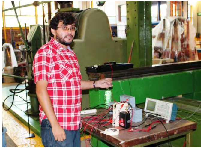
Figure 4. Optical interrogation and data acquisition system installed at the mechanical test laboratory.
