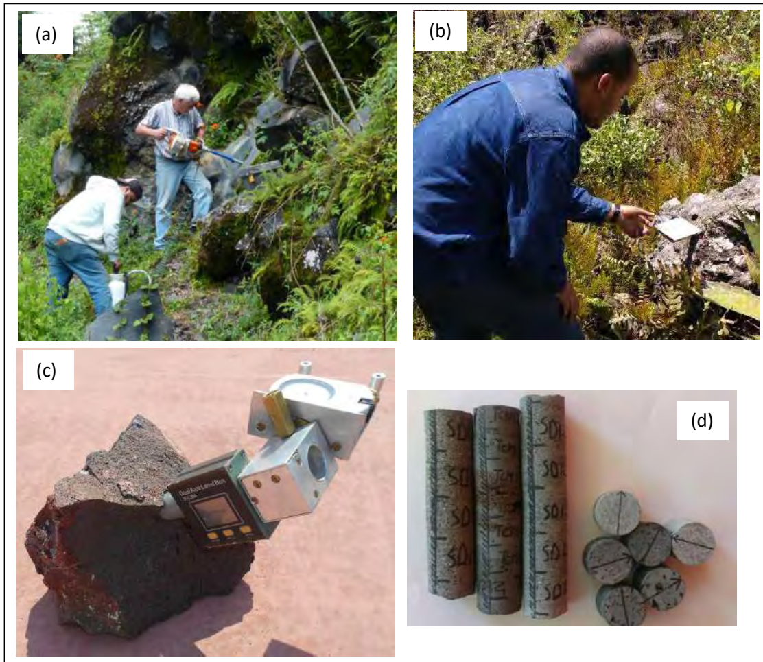
Figure 1.4 (a) Field sampling image showing how we drill the lava flow using portable gasoline-powered drill; (b) Another image demonstrate how we orient the samples before taking out from the attached rock outcrop; (c) Overall view of the orienting device used in the present thesis with digital inclinometer and sun to magnetic compass with ocular reading; (d) Paleomagnetic core samples with the orientation arrows, and also showed some specimens.
