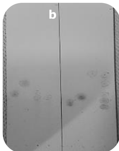
Figure 2. Thin layer chromatography plate with mixture of simple sugar standards and two samples of mucilage (from left to right): a) arabinose, xylose, mucilage 1 and mucilage 2; b) galacturonic acid, galactose, rhamnose, all standards.
