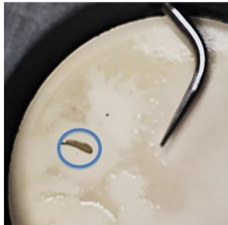
Figure 4. Damaged surface of a 0.8 μm ceramic membrane produced by a UDS tip 10P exceeding the exposure time (longer than 30 minutes).
