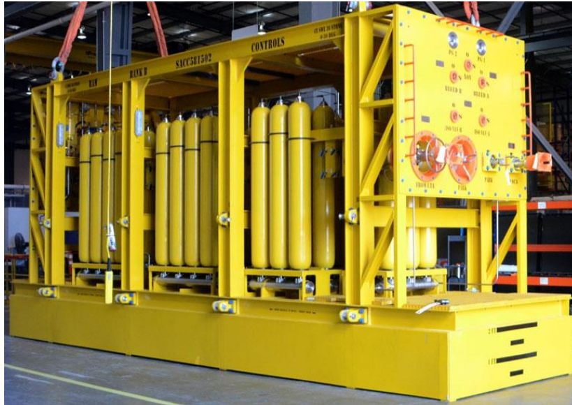
Figura 9 Acumulador Submarino, Marine Well Containment Company.
