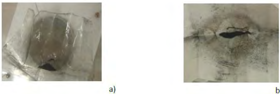
Figure 23: a) Airborne particles gathered in a plastic foil, b) Airborne particles gathered in teflon foil. The airborne particles are seen as a black fine powder.
