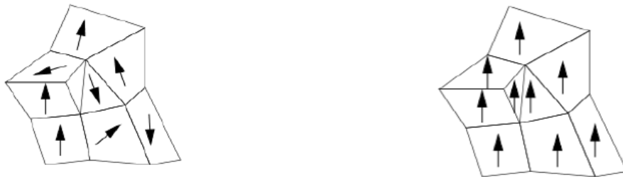
Figure 2: Visual representation of the magnetic moments in a grain. Lines represent the boundaries of the domains, arrows represent the direction of the magnetic moments in each domain. On the right grain, the magnetic moments remain aligned after an external field was applied. (Hughes, 2005).
