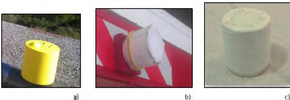
Figure 16: a) Latex cover from location U 2 , airborne particles are not appreciated. In b) filter paper cover from location U 1 from the separated area; airborne particles are appreciated around the magnet's diameter edges as a fine black line of dust. In c) teflon tape cover, magnetic particles are not appreciated.
