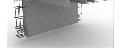
**D-10 DETALLE DE EMPOTRE DE PLACA TT CON VIGA PRETENSADA**
