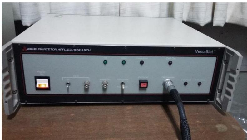
Figura 1.8 Potenciostato VersaStat I. EG & G Princeton Applied Research.
