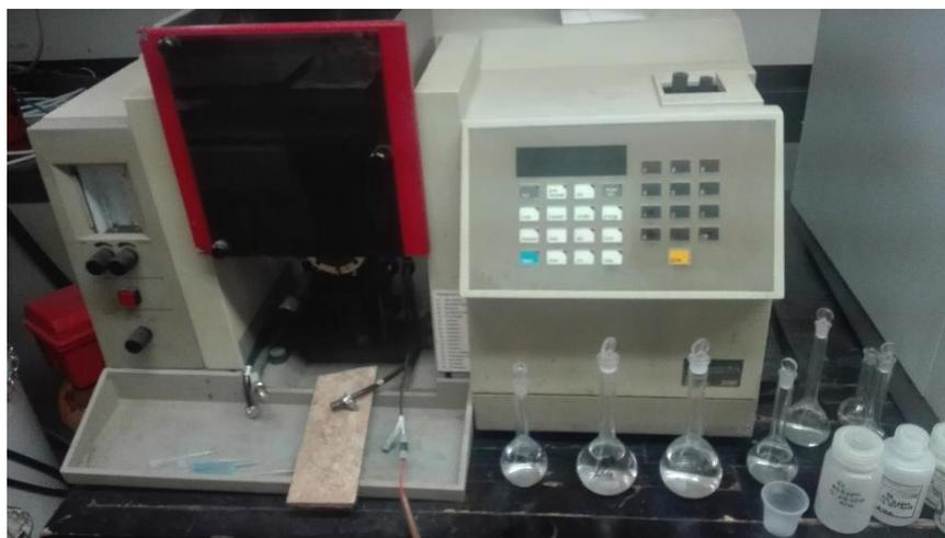
Figura 2.3.3 Atomic Absorption Spectrometer (AAS) Modelo Perkin Elmer 3100.
