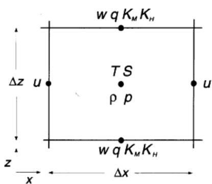
Fig. 3 — Vertical layout of variables on model grid
