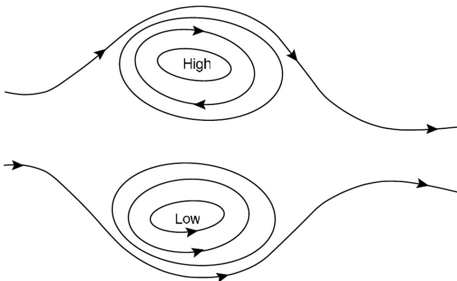
**Fig. 2.5** Schematic of geostrophic flow with a positive value of the Coriolis parameter  $f$ . Flow is parallel to the lines of constant pressure (isobars). Cyclonic flow is anticlockwise around a low pressure region and anticyclonic flow is clockwise around a high. If  $f$  were negative, as in the Southern Hemisphere, (anti)cyclonic flow would be (anti)clockwise.
