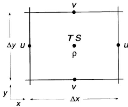
Fig. 1 — Horizontal layout of variables on model grid
