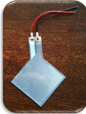
*Fig. 1.10 Transductor de material PVDF [17]*
