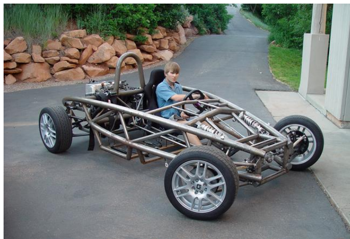
Fig. 1-6 Chasis espacial tubular [16]
