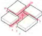
MASSING & PROGRAM ORGANIZATION Programs are organized vertically to retain all required adjacencies and visual permeability in a compact volume. The program is organized by an irregular volume, which is then carved around a central atrium as an organizing principle.
