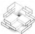
SETBACKS & WINDOWS This system of setbacks and setbacks is repeated on the upper floors. The setbacks create the volumes around to create space for windows that are removed from the street, increasing privacy and security. They also accommodate mandatory residential and office requirements.
