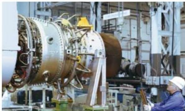
**Figura 87:** Generador SGT-100 (Fuente: <http://www.energy.siemens.com/hq/en/fossil-power-generation/gas-turbines/>)
