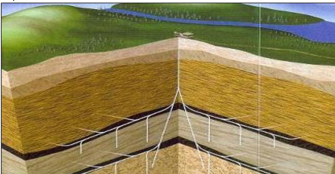
**Figura 36.** Pozos multilaterales. Fuente: Target Drilling “Precision Drilling for Your Success” (2014) Recuperado de: <http://www.targetdrilling.com/surface-cbm.html>
