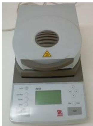
Figura 9. Termobalanza OHAUS MB-45.
