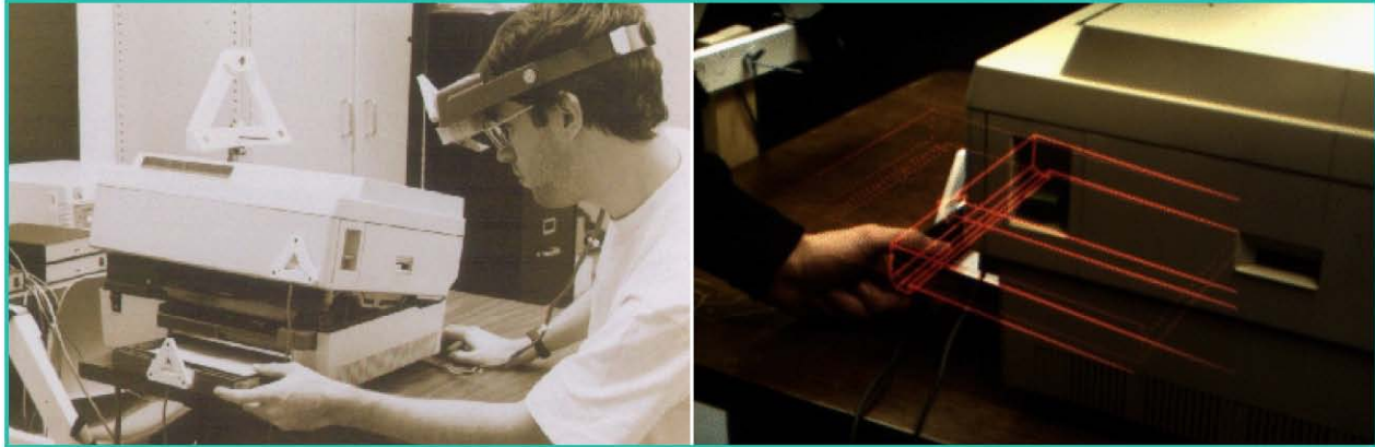
Imagen 8. KARMA (Knowledge based Augmented Reality for Maintenance Assistance). Recuperada de : http://www.augmentedrealityvisor.com/
