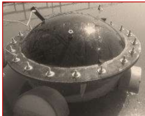
Figure 4.5. A view of the static chamber used in this study (five similar units).
