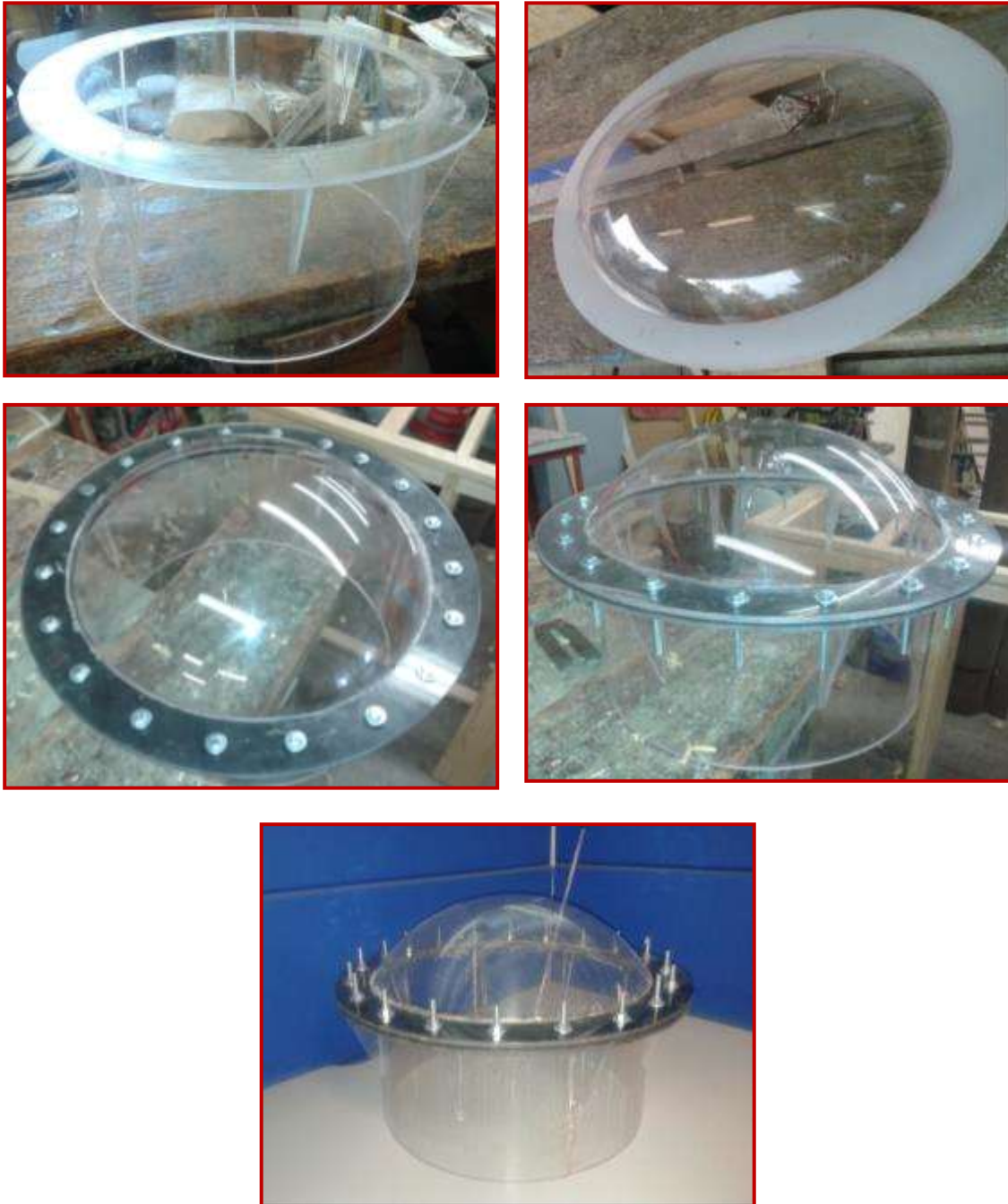
Figure 10. Assembly of Static Flux Chamber.
