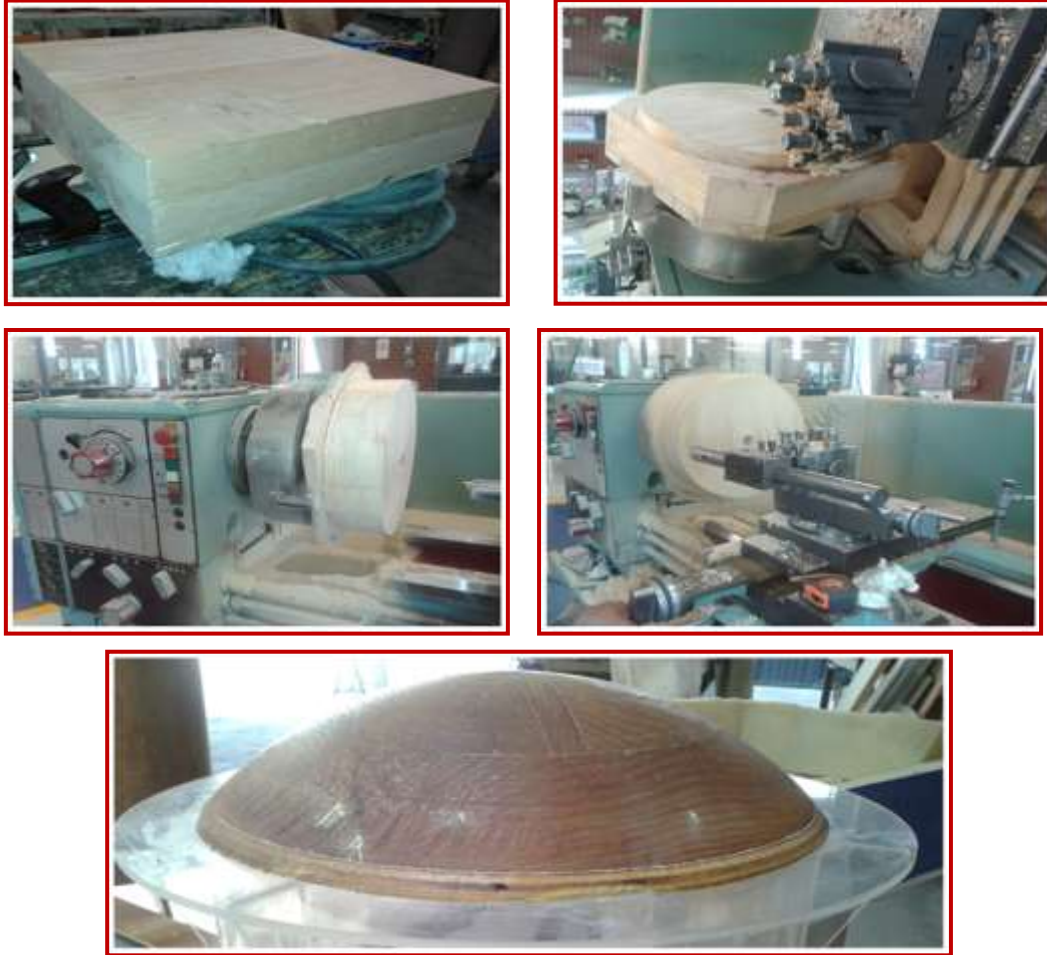
Figure 9. Making of the wooden mold for the dome of the Static Flux Chamber.
