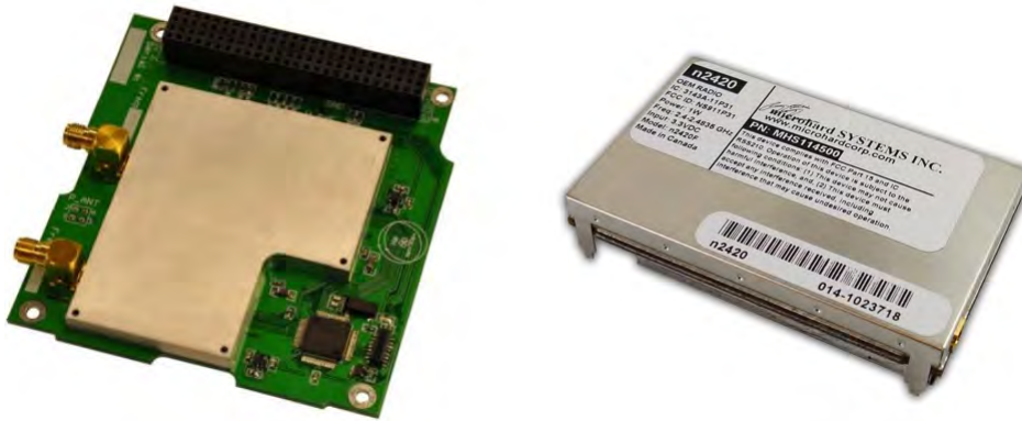
Figura 2.4: Astrodev He-100 y Microhard n2420
