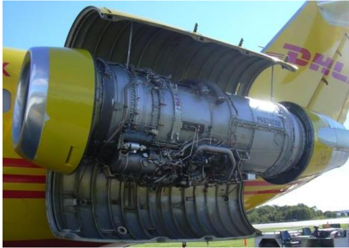
Figura 1.6 Turbo fan [low bypass] Pratt & Whitney JT8D, (KPWM Spotter 2004)
