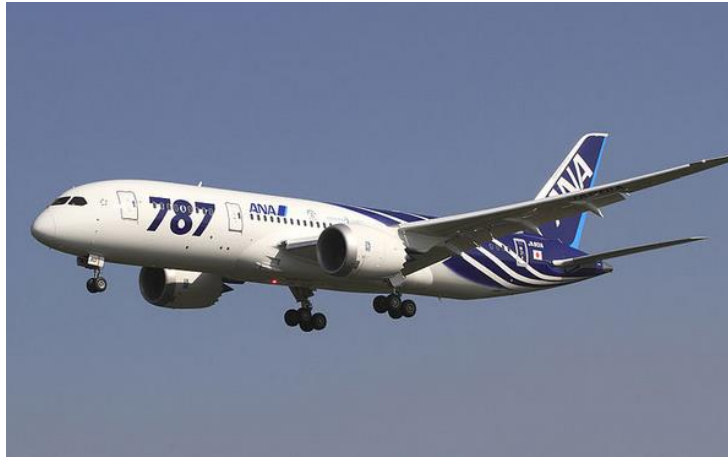
Figura 1.7 Aero nave con Turbo fan (high bypass) Boeing 787, (All Nippon Airways Boeing 787-8 Dreamliner JA801A 2013)
