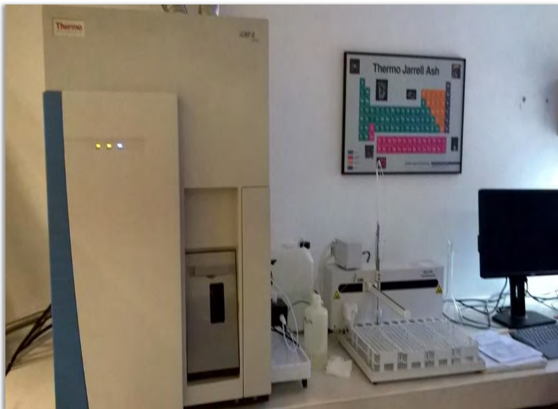
Figura 9 ICP-MS iCAP Q
