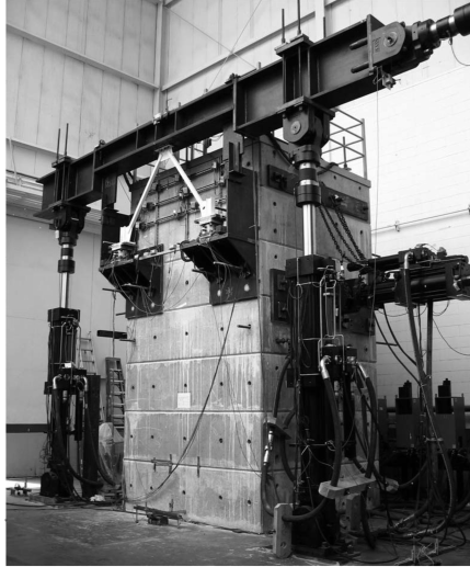
Figure 3.10: Actuators configuration for a V-Brace testing.
