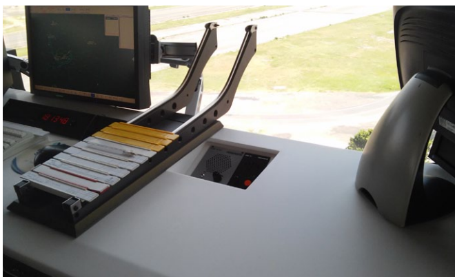
Figure 39: Reduced space due to the clock and the strip rack in the Helicopter console.
