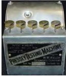
**Figura1. Pressey Testing Machine.**
