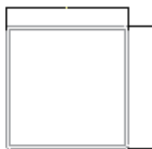
COLUMNA C-1 HSS 12" X 12" X 3/8" W=85.45 KG/ML
