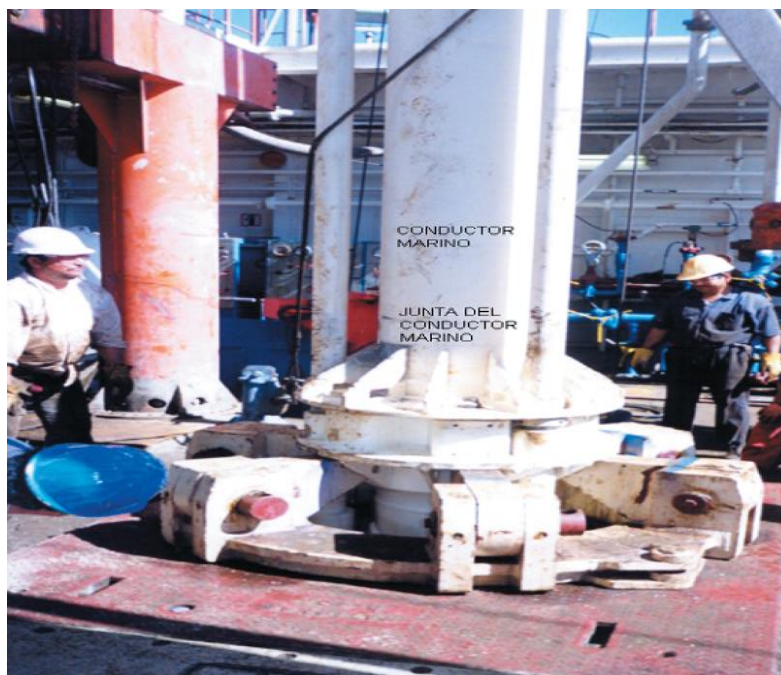
FIGURA 17. CONDUCTOR MARINO (RISER)
