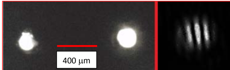
Figure E.2. Left panel: photograph of the manufactured slit. The image shows two apertures of about 200\mu\text{m} separated a distance of 800\mu\text{m} . Right panel: diffraction pattern generated by green laser light passing through the custom made slit. It is clear from the fringe patterns that the slit effectively diffracts the light passing through the slit.
