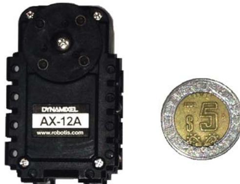
Figura 3.3: Servomotor AX-12
