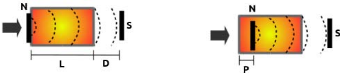
Fig. 3.3.2: Schematic drawings of the two PVA-phantoms with a 1.5 mm thick slice of neoprene ( N ) inside. Left: N is positioned at the very extreme of the probe to gain superficial photoacoustic response. Right: N is shifted 1 cm ( P ) inside.
