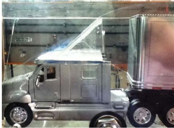
Fig. 5.26 Deflector de aire a 41° a 3 m/s
