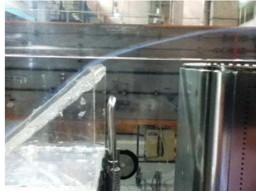
Fig. 5.27 Deflector de aire a 41° a 4 m/s
