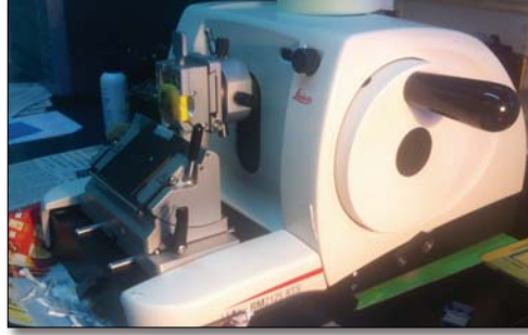
Figura 19. Microtomo Leica RM2125 RTS.
