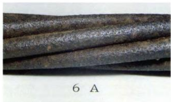
Photo 6A. Strand surface after cleaning.
