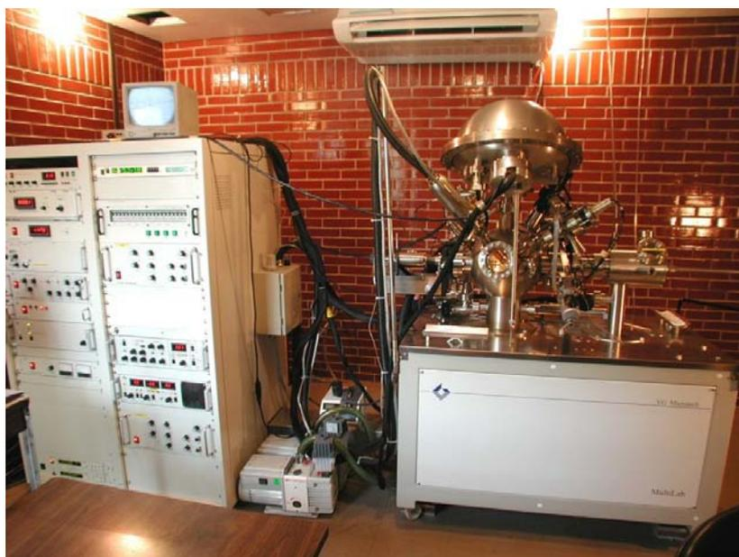
Figura 2.8: Sistema VG Microtech ESCA2000 Multilab UHV.
