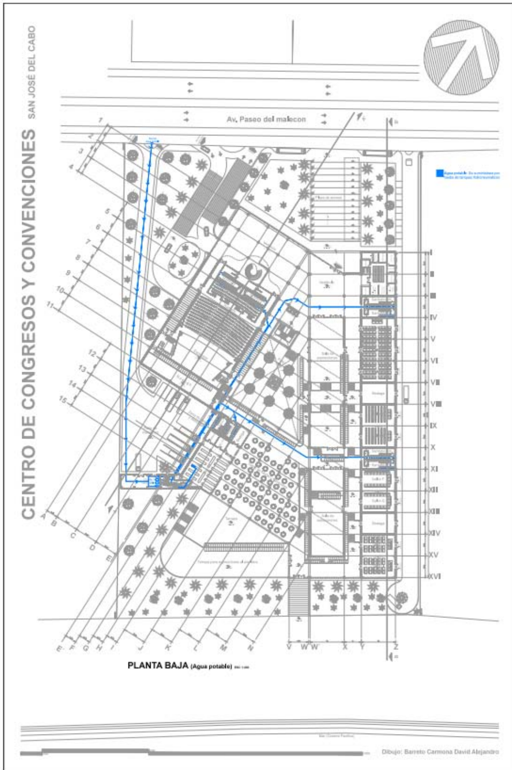
PLANTA BAJA (Agua potable)
