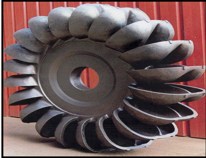
Figura 1.21. Rotor de turbina Pelton, (Faeitch, 2011).
