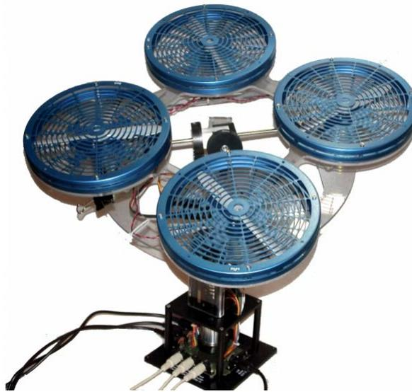
**Figura B.1:** Plataforma experimental Quanser 3DOF Hover
