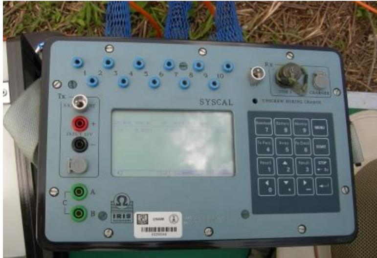
Figura 4.3 Resistivímetro SYSCAL Pro Switch de Iris Instruments.
