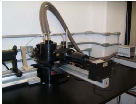
**Figura 9.** Dispersor de Luz, Marca Brookhaven Instruments Corporation, Modelo BI-APD
