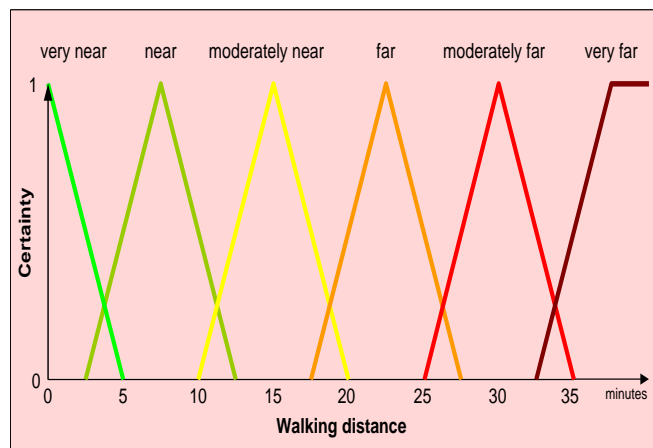
Figure 4.5 Fuzzy functions for different proximity relations measured as walking distance in minutes with their corresponding certainty or membership values.
