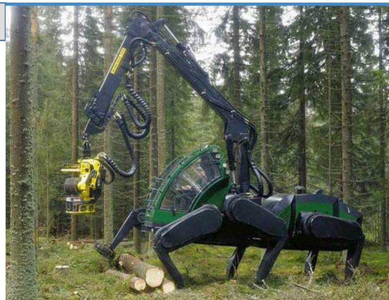
Fig. 1.23 Timberjack Walking Machine.
