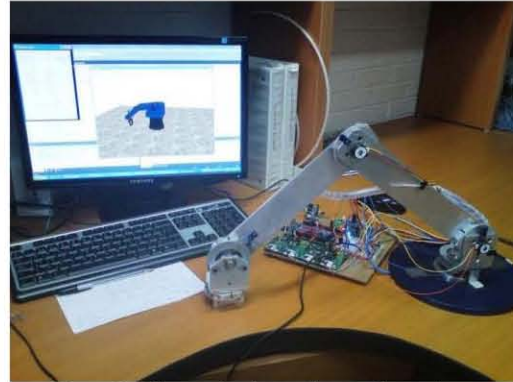
Figure 13. Teleoperation System for experimentation
