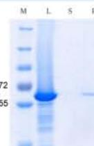
Fig. 5. Fractions of laccase reaction with 4-MeOPh. Native laccase (L), supernatant fraction (S) and polymer fraction (P).
