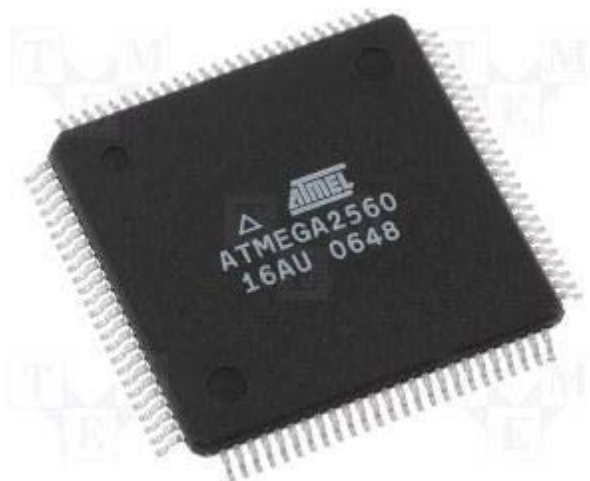
Figura 4-69: Miroposador ATmega2560 ( http://atmega2560-16au.katalog-tme.pl )
