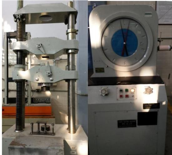
**FIGURA 13. Prensa universal (Tokio Testing Machine NFE Co, LM2)**
