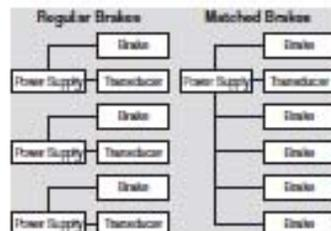
To solve this problem, Magtrol developed a system to assure that every brake of a given model designation will be matched—at a predetermined torque and current
