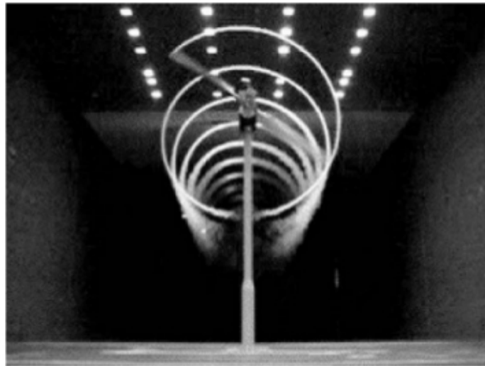
Figure 1.4: Flow visualization with smoke generated in tip, revealing smoke trails for the NREL turbine in the NASA-Ames[24]
