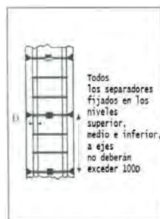
Figura B.84 – SEPARADORES A LO LARGO DE COLUMNAS - Fuente: Preparing for Quality, Site Supervisors Guide, The Ready-mixed Concrete Bureau, 1995, p. 80
