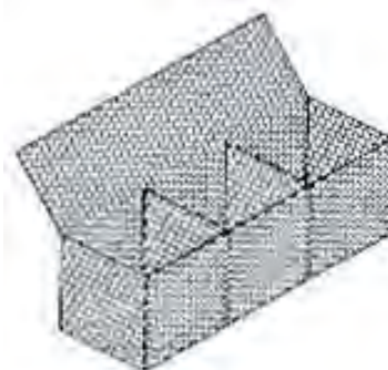
III – Gavión con 2 diafragmas Handbook of Slope Stabilisation, J.A.R. ORTIGAO y A.S.F.J. Sayao Editors, Edit. Springer, 2004; p. 234
