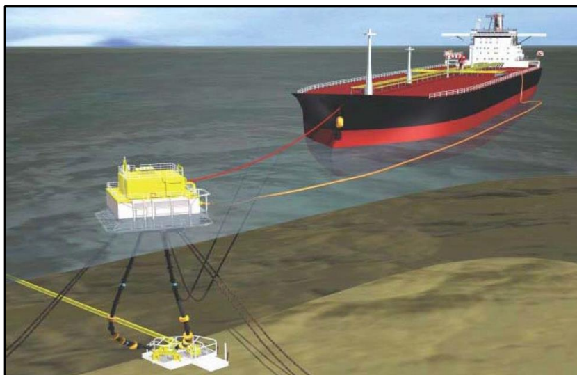
Figura 2-17 Transferencia de aceite Single Point Mooring (SPM). ( www.shipswiki.com )
